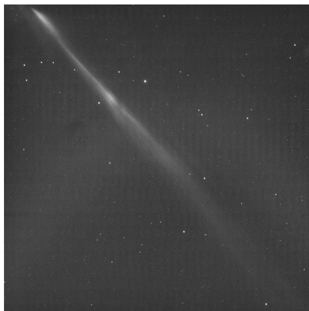
Fig. 18. Example of diagonal streak from stray light in a NAC image (N1472601232). This streak is produced by the satellite Tethys, which lies less than 1/2 of a NAC FOV off of the upper left corner of this image.
